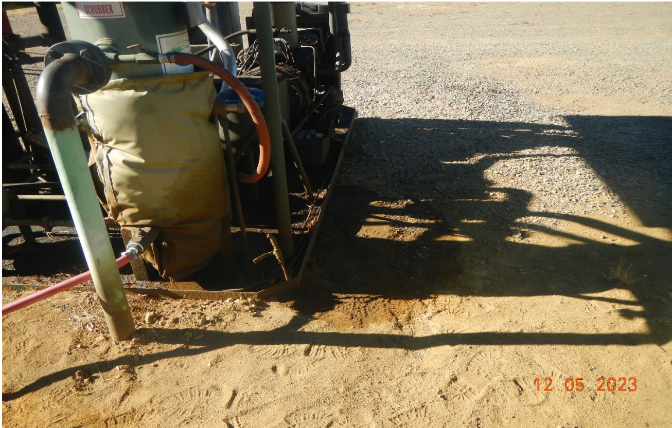
Photo 4. There is stained soil next to the engine skid that will need to be cleaned up.
