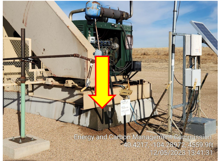
Photo 2 – Stained Soil at Gas Engine
