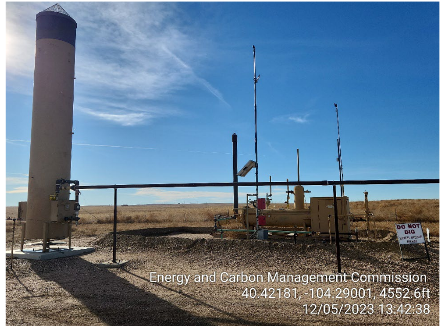
Photo 4 – Separator and ECD
