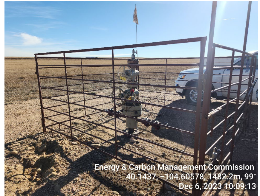
Photo 2: TA wellhead
