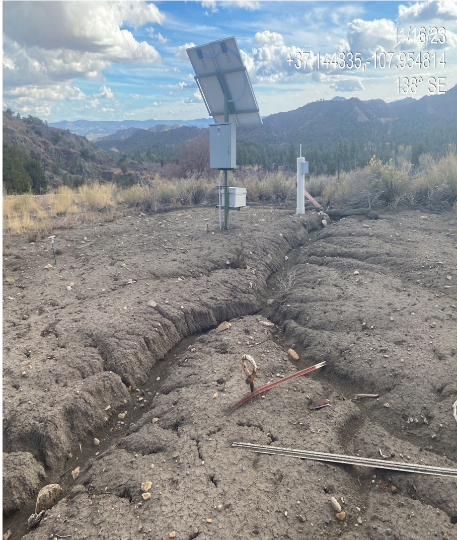
Photo 4. View of rill erosion and failing stormwater BMPs observed in the southern interim area of the disturbance.
