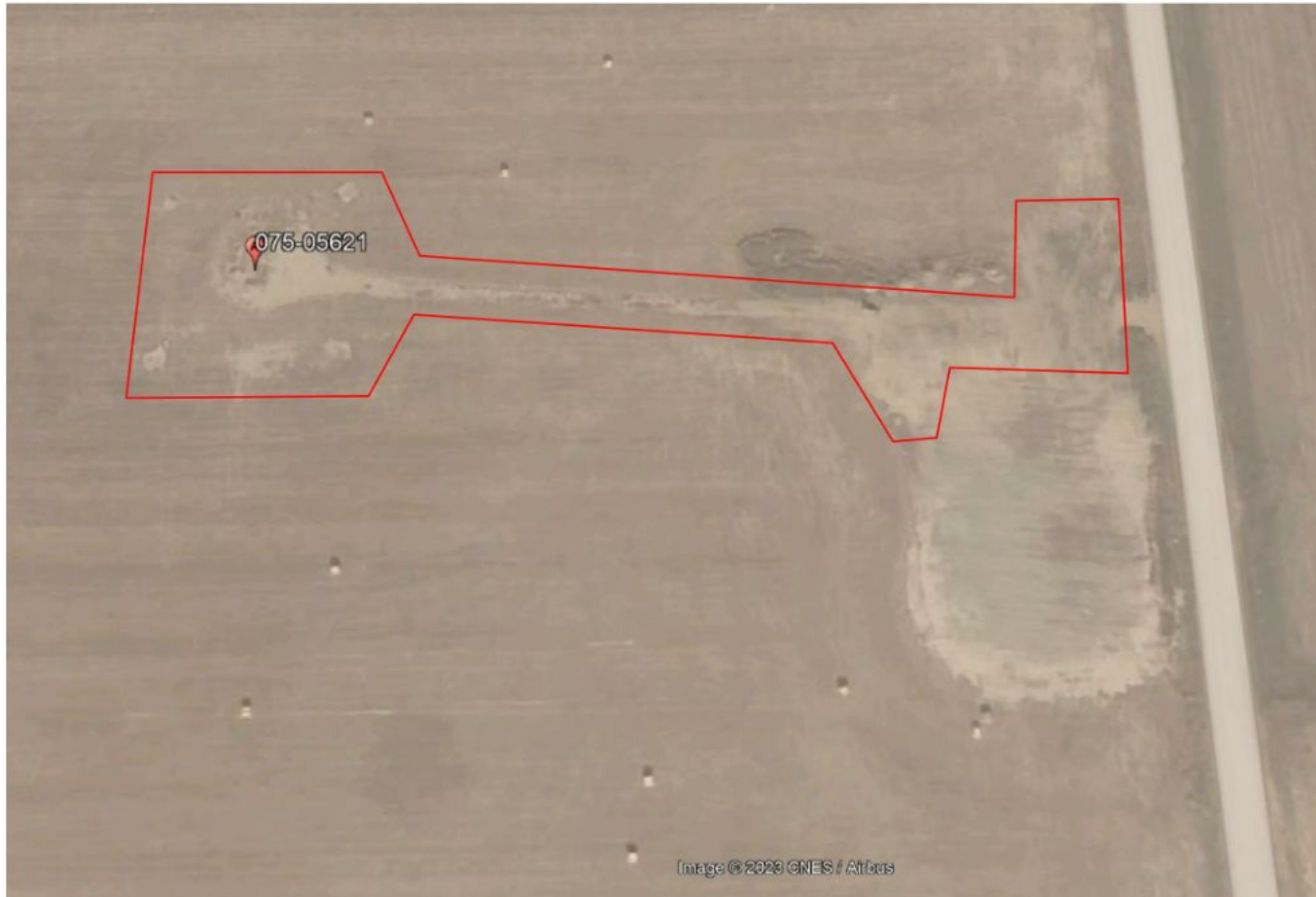
Photo 11. Google Earth aerial imagery (circa 10/2020) illustrating red outline of former access road, well location, and production area disturbances that will require final reclamation activities ASAP. Active remediation should not preclude the commencement of final reclamation activities on the above identified areas. Final reclamation should have been completed by 07/22/2019, per 1004 Rules.
