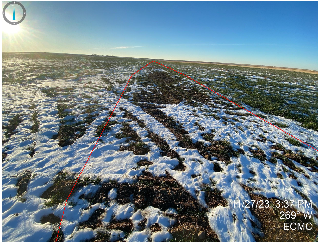
Photo 7. Taken from the northwest corner of the former production areas, where the well access road starts. It is apparent that no reclamation work has been conducted since the previous inspections. Gravel/road base material remain on location and requires removal to comply with Rule 1004.
