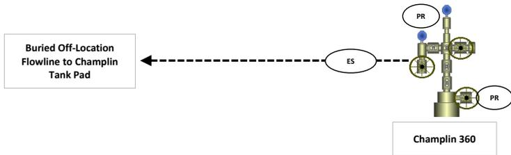
NOTE: This well is a conventional vertical well. No stimulation will be required to complete this well, therefore no flowback will be required. All formation fluids will be separated with a 3-phase separator. Produced water will be trucked to disposal at a commercial UIC well and condensate (if any) will be sold to an oil purchaser. All gas will be sent to the Ladder Creek Gathering System operated by Tumbleweed Midstream for processing.
