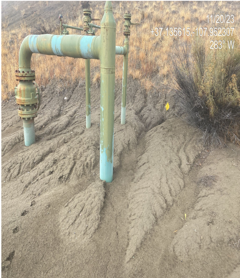
Photo 3. Rill erosion observed in the northern interim reclamation area at the base of the cut slope.
