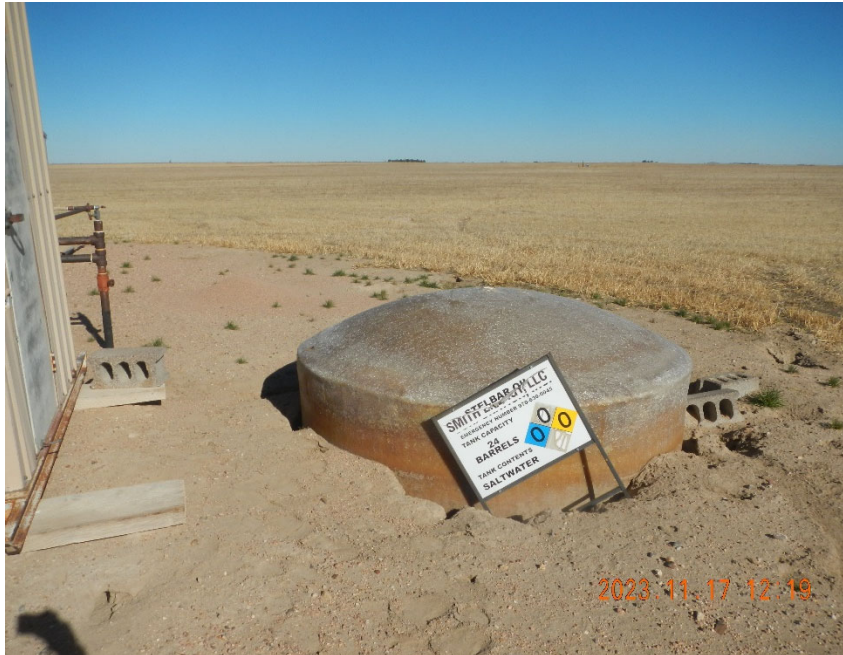
9. Produced water tank at remote gas meter run.
