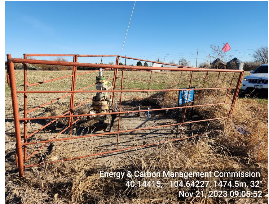
Photo 2: TA Wellhead, WEEDS, fencing in disrepair
