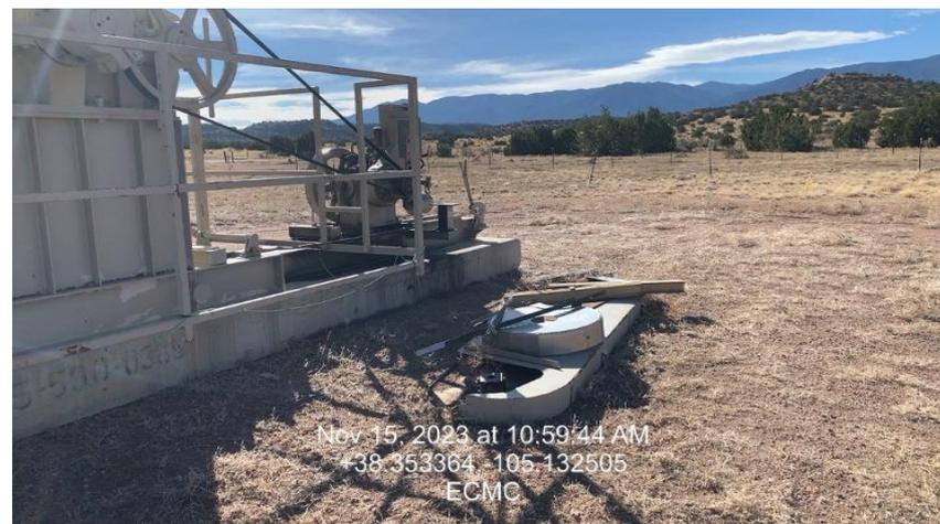
**Photo 7 – Evidence of oil leak on Pumping unit, Unit appears to be down for maintenance**
