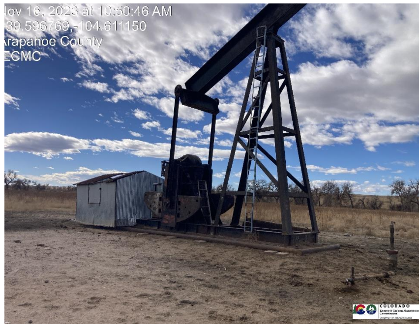
Pic 1 wellhead / pump jack
