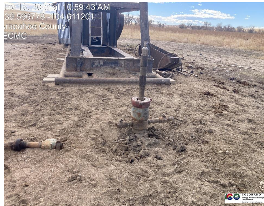
Pic 2 bradenhead is not plumbed to surface.
