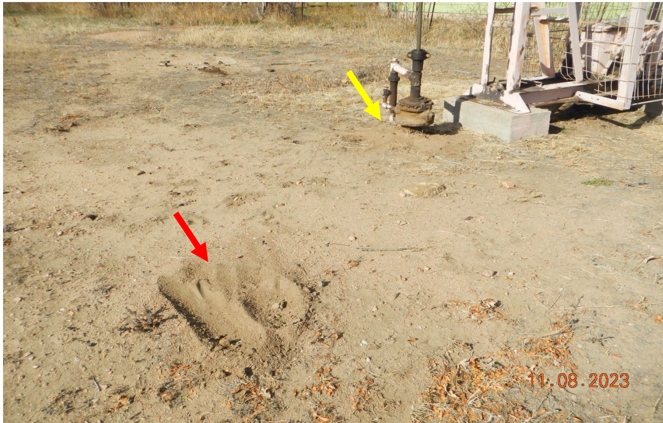
Photo 3. Facing toward the well. It appears soils was scooped up at red arrow to cover oil stained soil at the wellhead. The oil stained soils need to be cleaned up and properly disposed.
