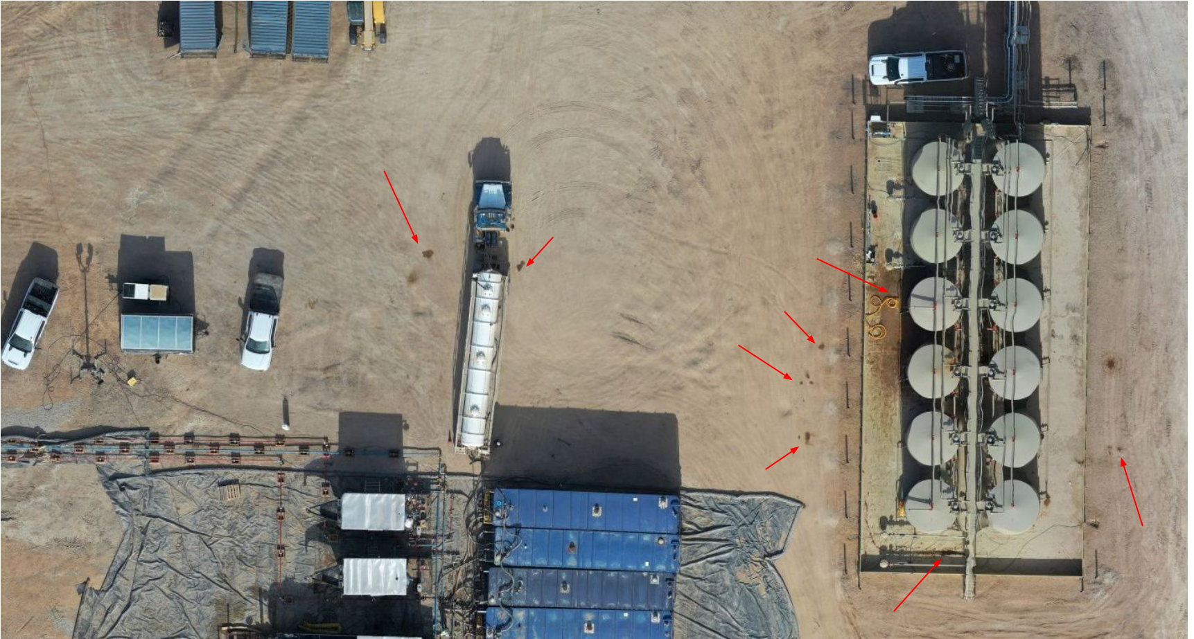
Photo 6. Drone aerial imagery illustrating stained soils throughout the production area and hydrocarbon impacts within the secondary containment of the tank battery.
