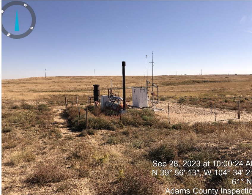
Photo #5 ECD, separator & meter house.
