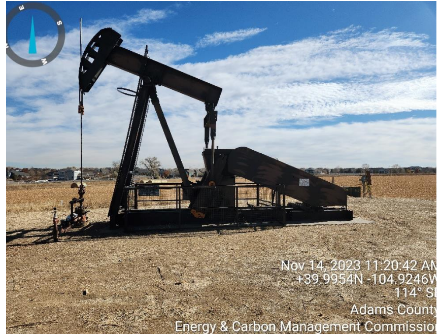
Photo 2 well head and equipment
