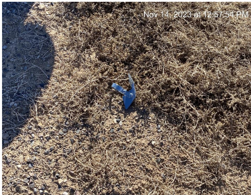
Rain cap off relief valve
