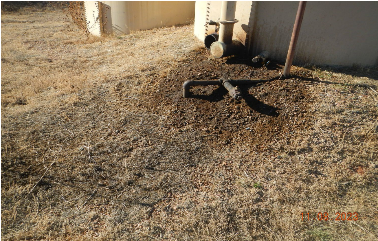
Photo 4. There is oil stained soils at the backside of the tanks.
