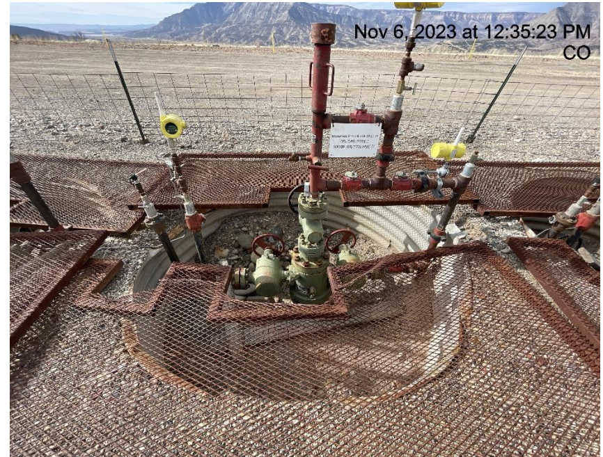
Photo # 5595 44A-08-07-95 Wellhead cellar lacks wildlife egress & cellar cover improperly placed & only partially covering cellar
