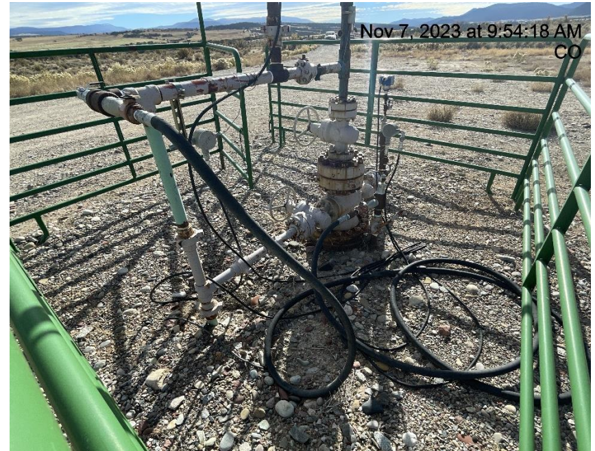
Photo # 5700 COUEY 8-3 bradenhead line connected to flow line.
