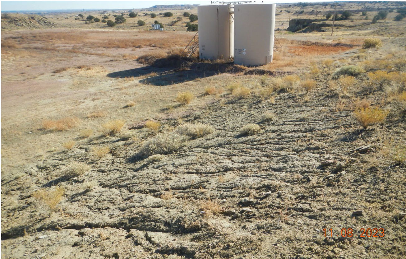
Photo 9. Facing east along the cut slope. There is rilling erosion along the cut slope.
