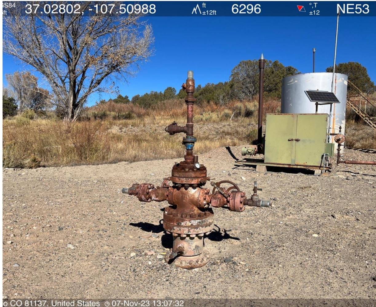
Photo #4 View of the wellhead assembly.
