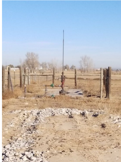
Plunger lift has been removed and converted to polished rod
