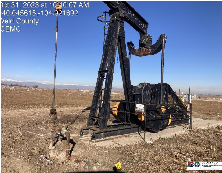
Pic 1 wellhead / pump jack
