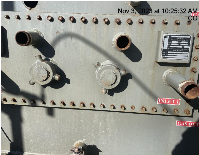
Photo # 5218 Open ended pipes on production separators/ wildlife hazard
