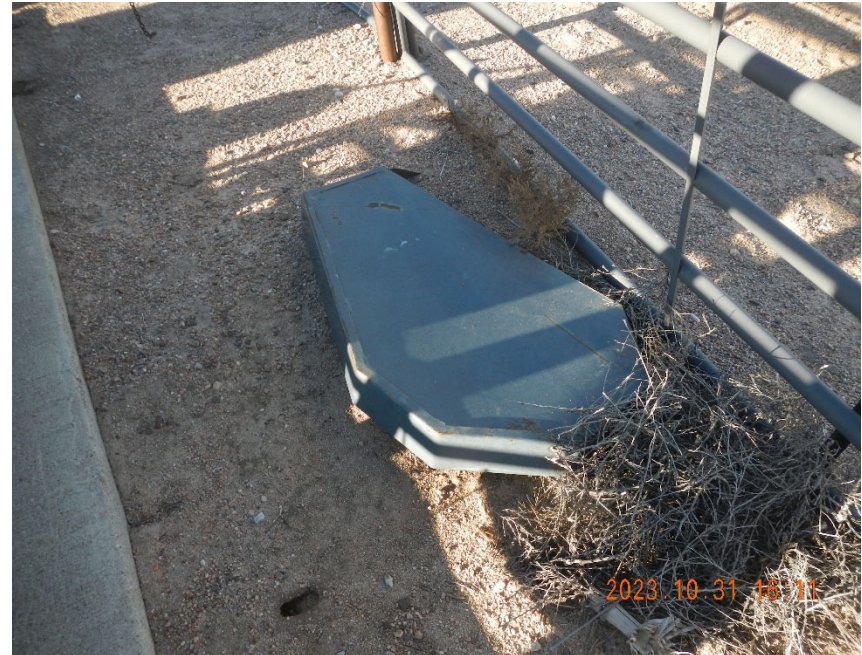
6. Pump Jack belt guard on ground inside fencing.
