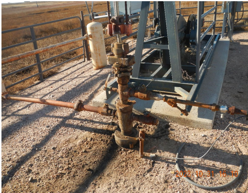
3. View of wellhead. Note staining around base of wellhead..
