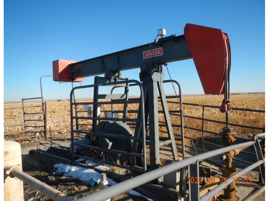
8. Pump Jack with stock panel safety barrier.
