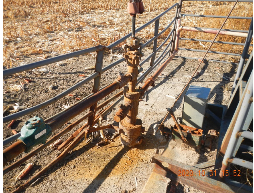
2. View of wellhead. Note staining around base of wellhead and damage stock panel..
