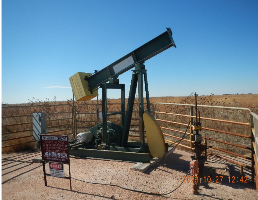
3. Pump Jack with Horsehead removed.
