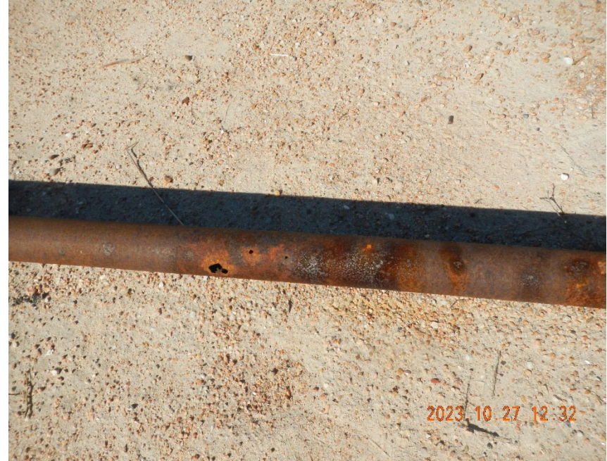
6. Holes along dump line to tank.
