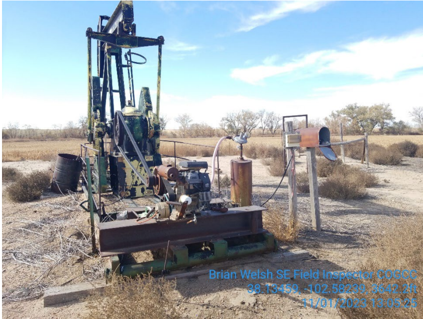
Prime mover and ancillary equipment
