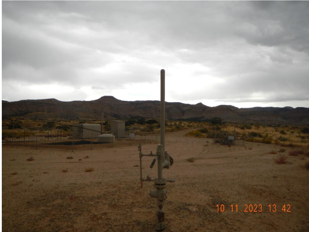
Unused flowline riser in south east corner of location.
