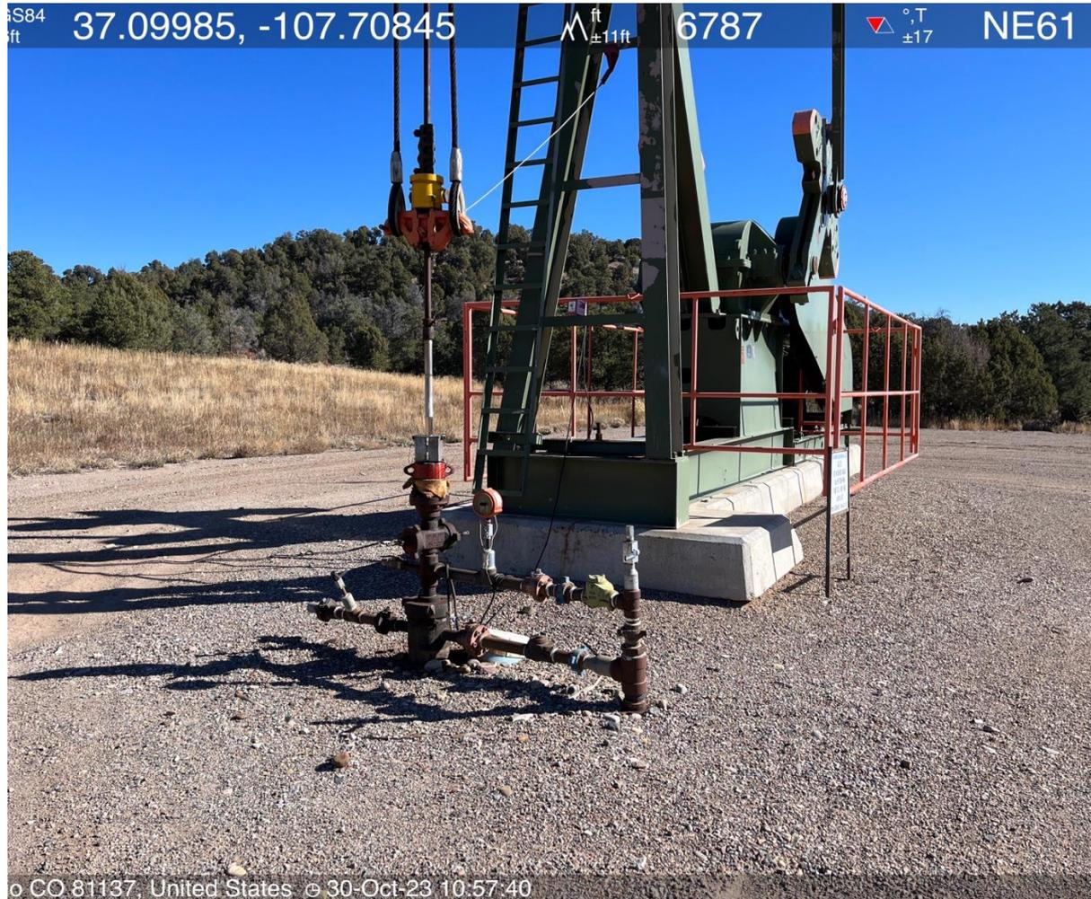
Photo #6 View of the IGE 135 wellhead and pumpjack.
