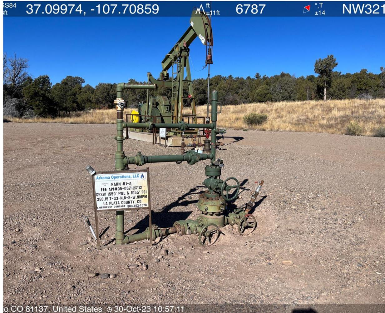
Photo #4 View of the Hahn #1-A wellhead assembly.
