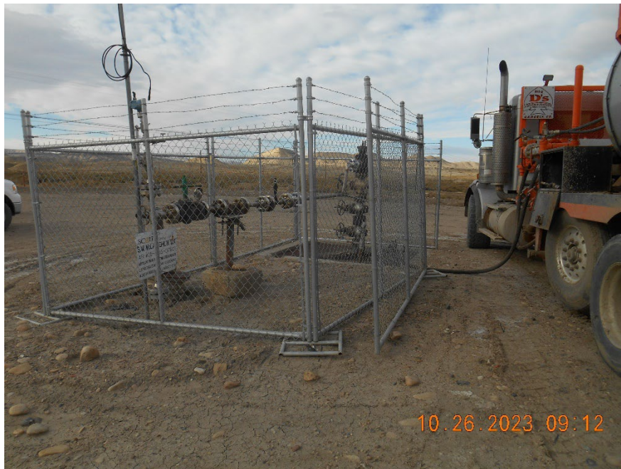
Injection well during MIT
