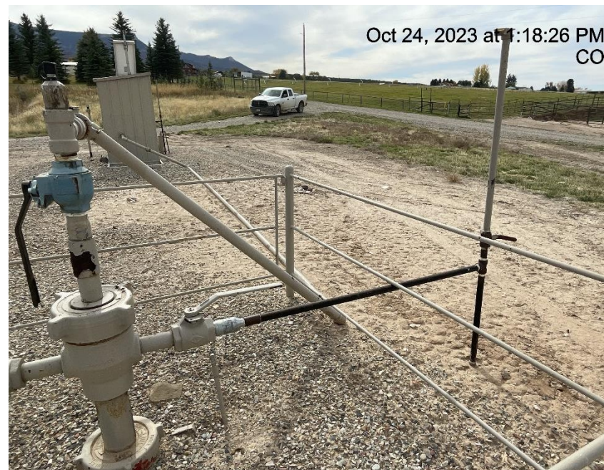
Photo # 4101 Domestic tap – 1 inch line coming off casing valve
