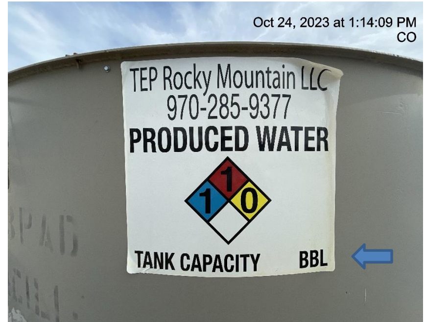
Photo # 4093 Tank label lacks required information
