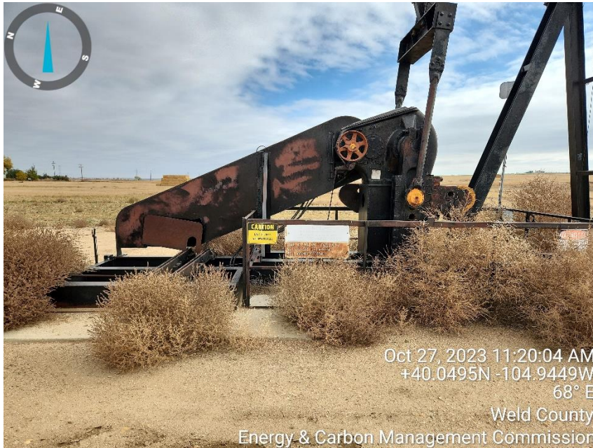
Photo 3 sign, missing motor, pumping unit
