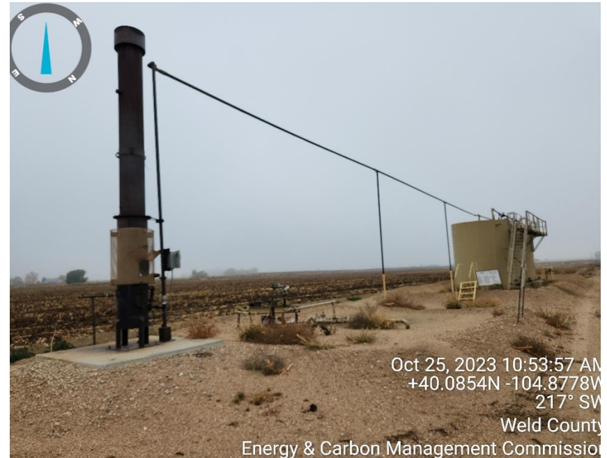
Photo 10 ECD and tank battery
