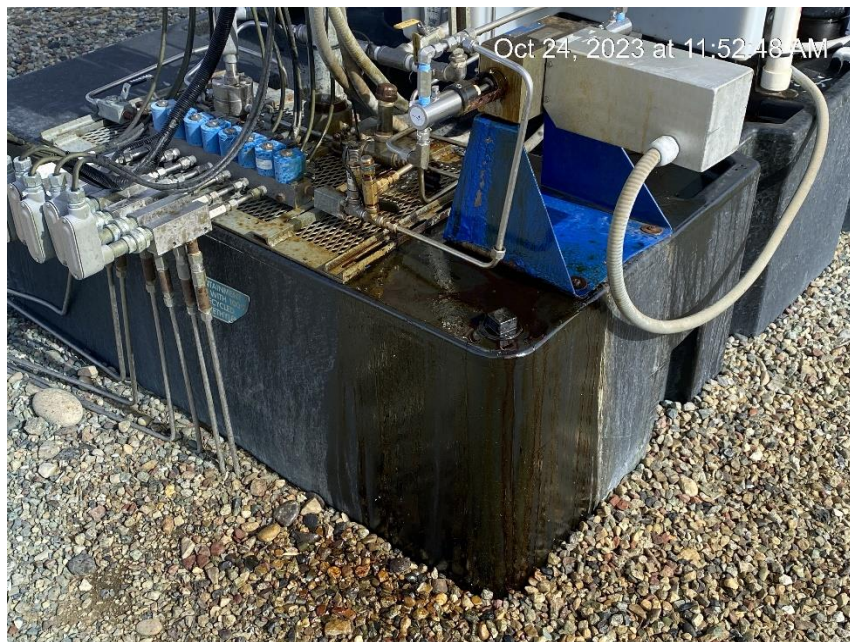
Chemical leaking on equipment and location
