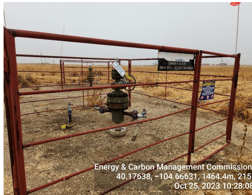
Photo 4: TA Wellhead
