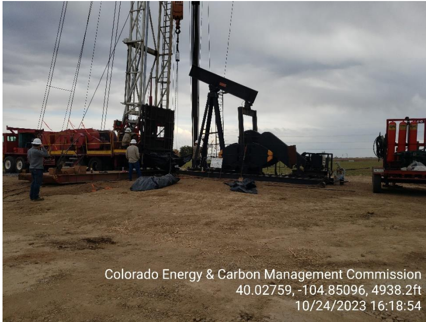
Photo 9 Rig 13 and pump jack set on well.
