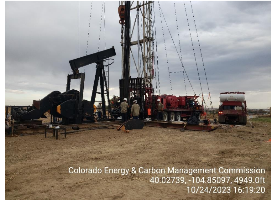
Photo 10 hot oil truck, rig and pump jack.
