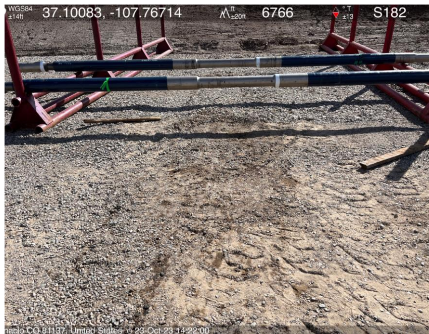
Photo #47 Impacted ground from leaky equipment.
