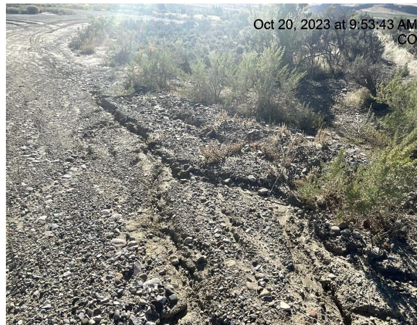
Photo # 3453 Erosion & transport of sediment off lease road into a vegetated area choking off vegetation/insufficient BMP's
