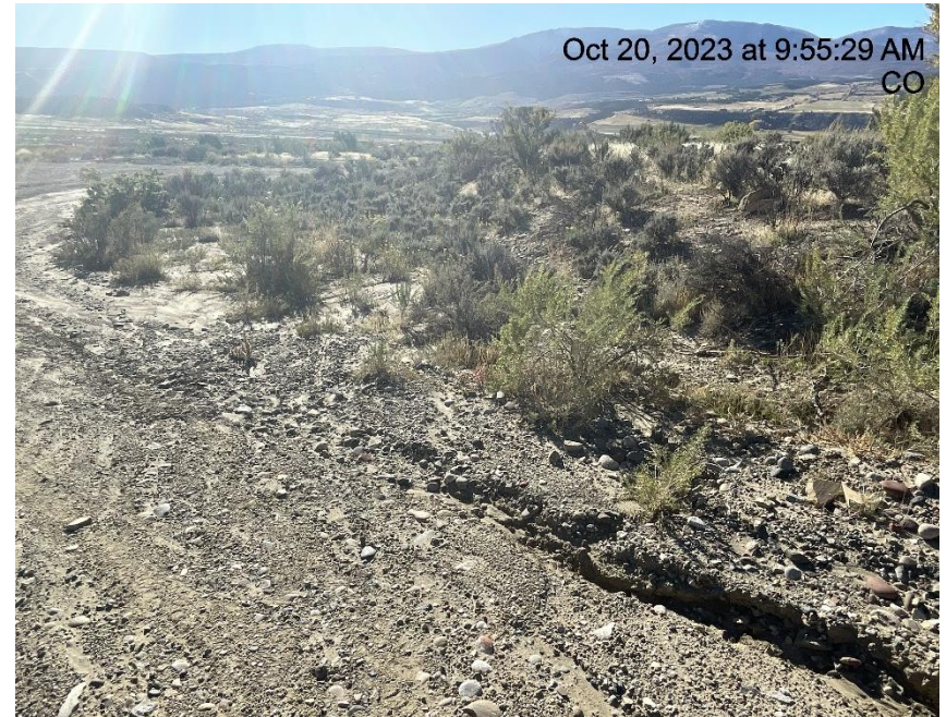
Photo # 3461 Erosion & transport of sediment off lease road into a vegetated area choking off vegetation/insufficient BMP's
