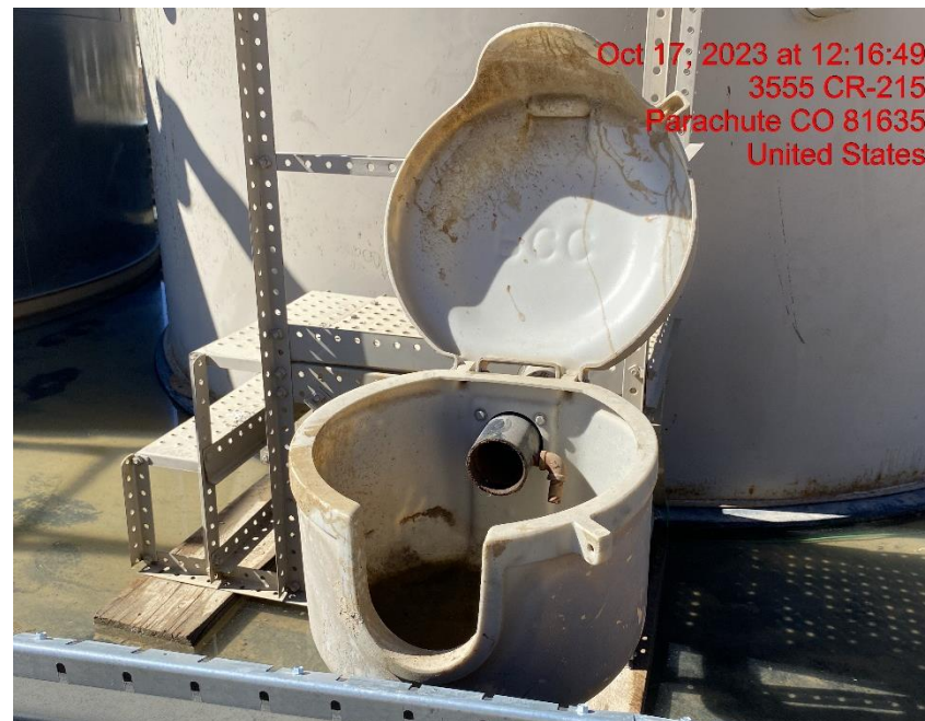
Open-Ended Load Line – Photo #07043
