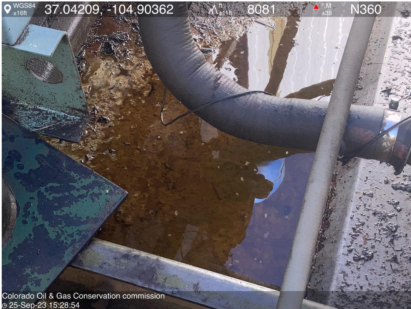
PHOTO 5: OILY WASTE IN ENGINE SKID. COMPLY WITH RULE 1002.f.(2)B, Comply with general provisions of the oil and gas act for wildlife protection AND SB-181. ca date 10-23-2023.
