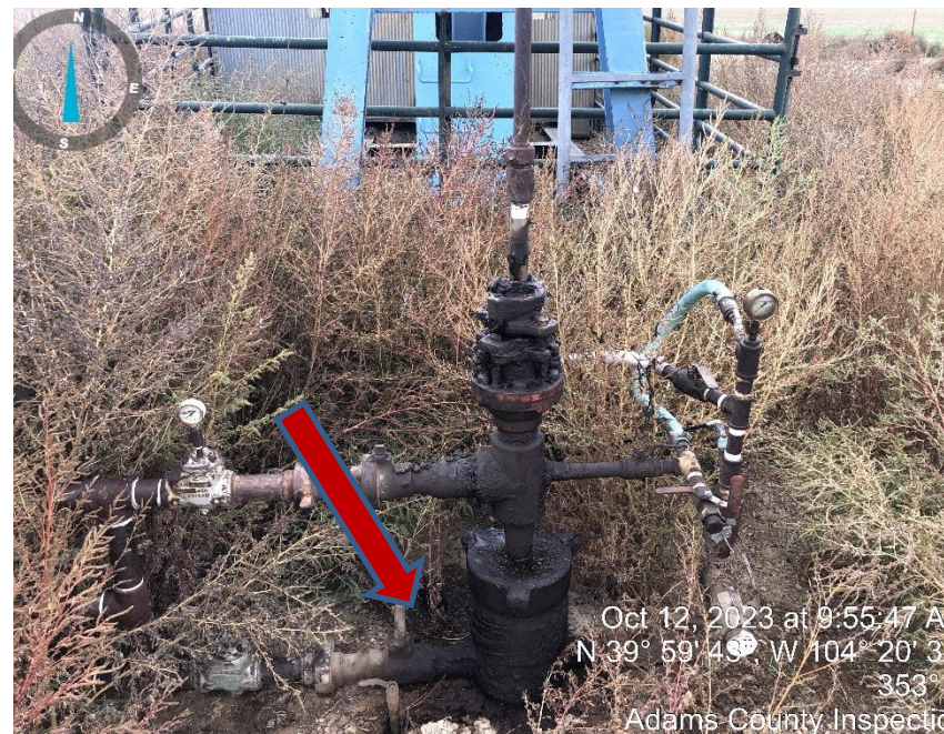
Photo #12 Stained soil around well head.
