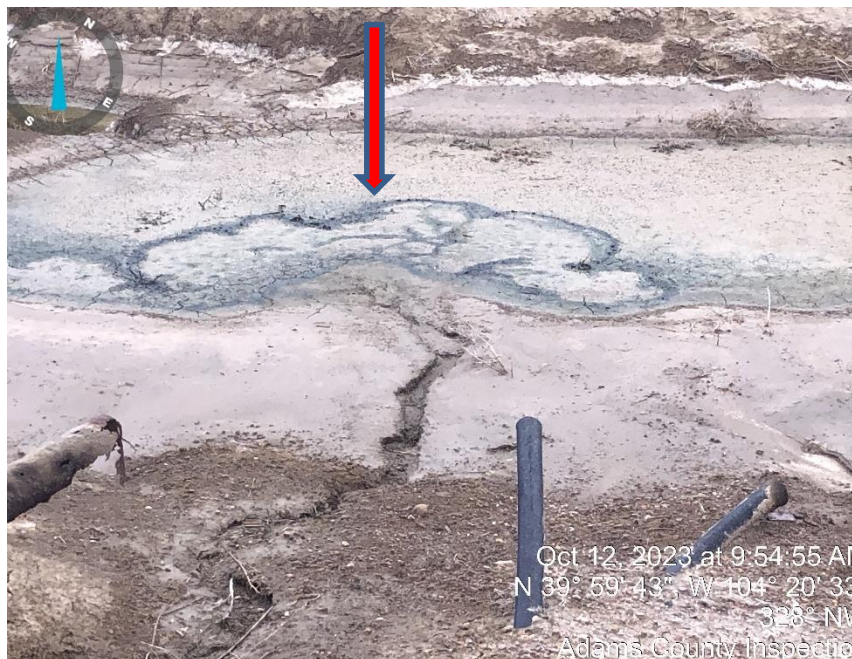
Photo #9 Hydrocarbons in the bottom of open pit.
