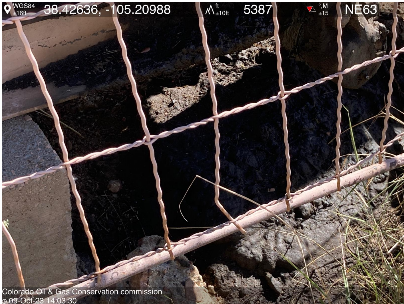
PHOTO 7: AREA OF IMPACTED SOIL UNDER PUMPJACK GEAR BOX. Conduct maintenance on equipment, cleanup stained material and review self inspection processes. COMPLY WITH RULE 1002,(2).D CA DATE 11-19-2023.
