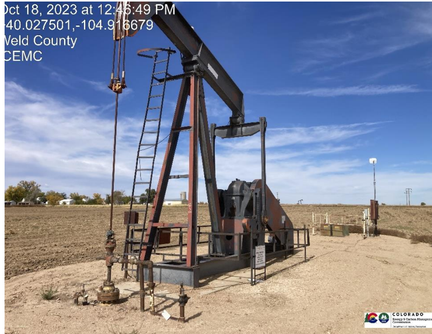
Pic 1 wellhead / pump jack
