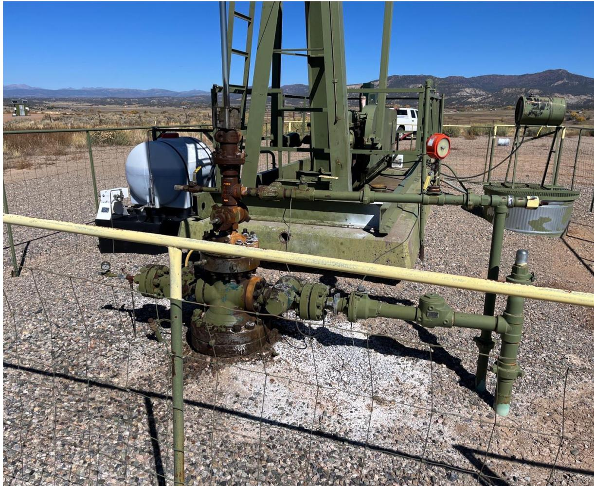
**Photo #4** View of wellhead assembly, impacted material on ground.
