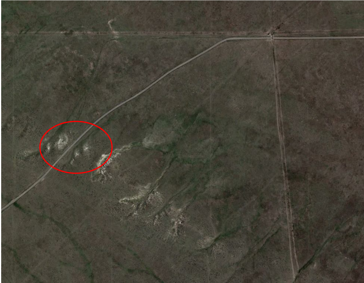
Photo 15. Google Earth aerial imagery from 7/17/2019 illustrates an area along the lease road where a BMP has not been properly installed and is not sufficient to control stormwater erosion off the lease road. Both Upland and CCRP will have to coordinate on the corrective action.
