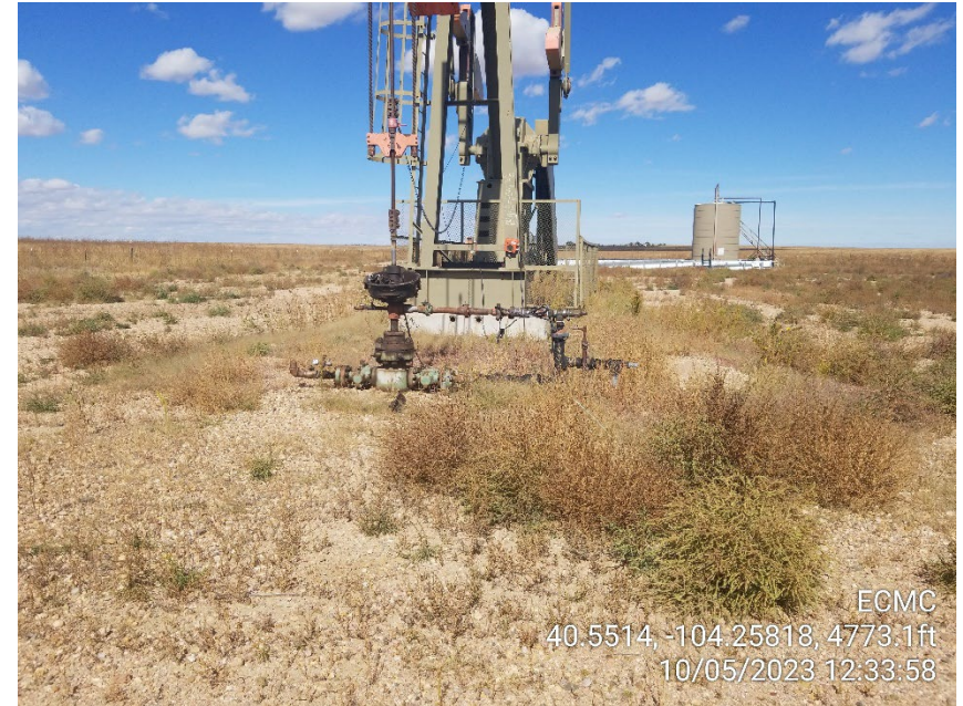
Photo 2 – Wellhead – Overgrown Vegetation and Stained Soil
