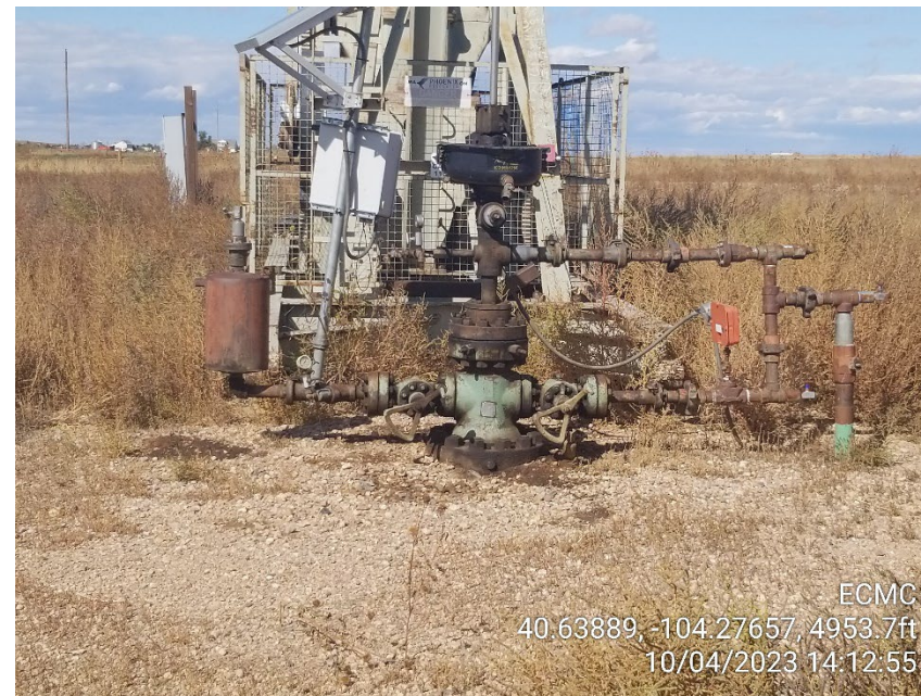
Photo 4 – Stained Soil – Wellhead
